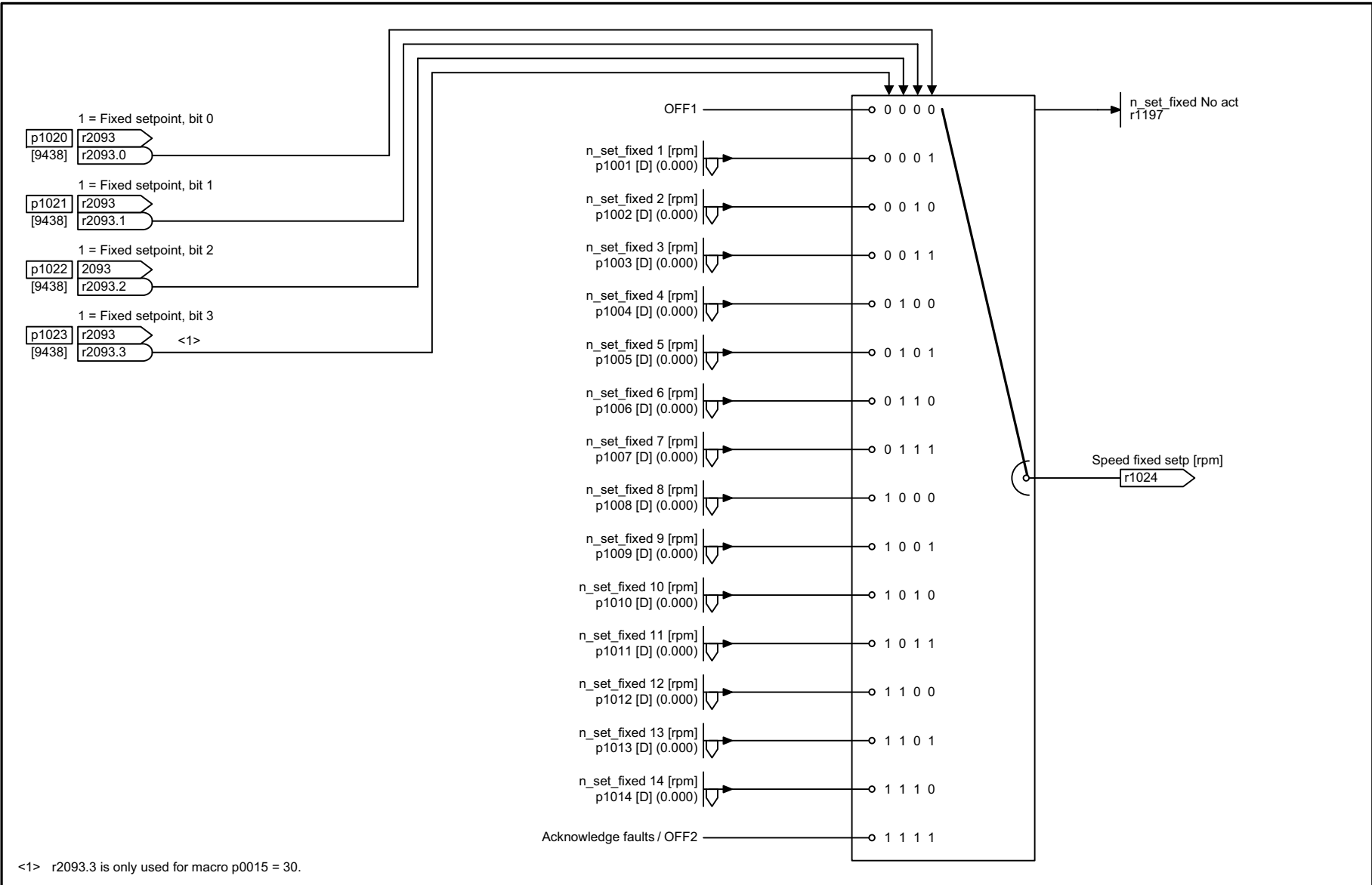
Fig. 3-38 9455 – Fixed speed setpoints (p0015 = 30/31, p1016 = 2)
