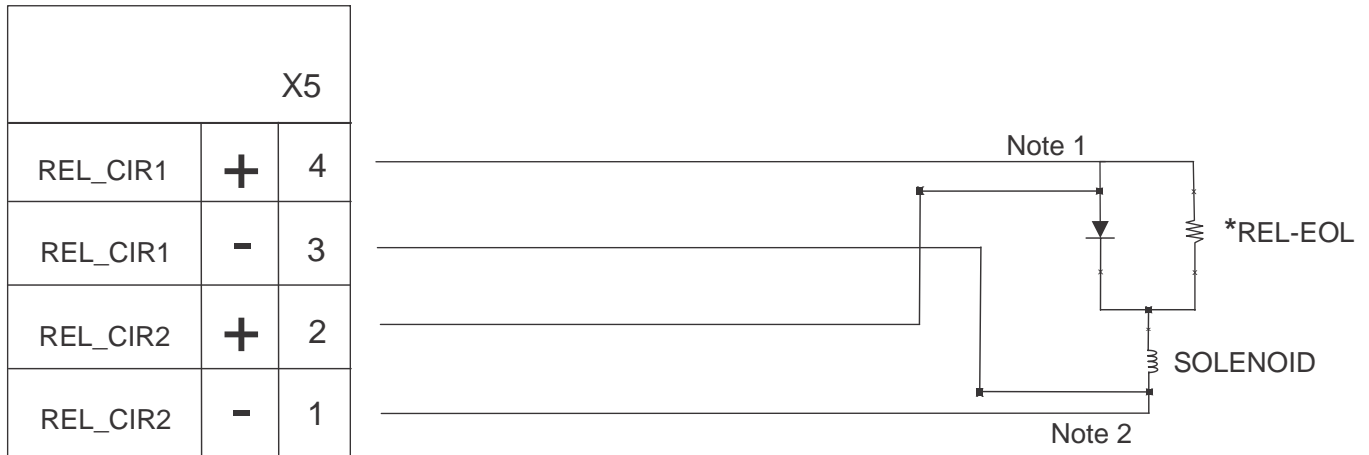
Figure 4: Class A wiring
