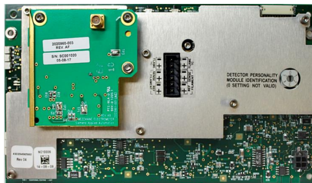
Figure 4. Base3 DPM shown with Mezzanine Module (A5E02645925001)
