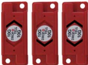
Figure 3-5 Shock indicator tripped
