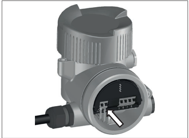
Fig. 10: Connection steps 5 and 6 - Double chamber housing
