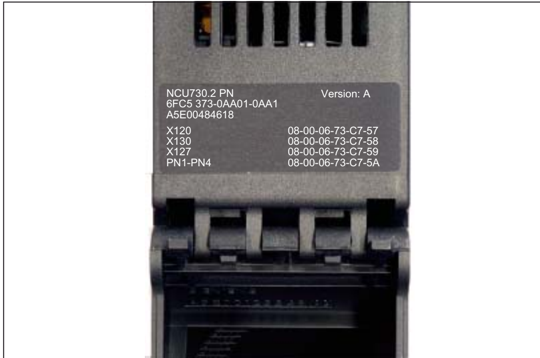
Figure 6-6 MAC addresses of the PROFINET/Ethernet interfaces
