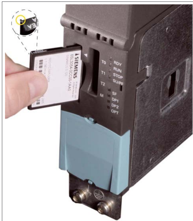
Figure 5-3 Inserting the CompactFlash card
