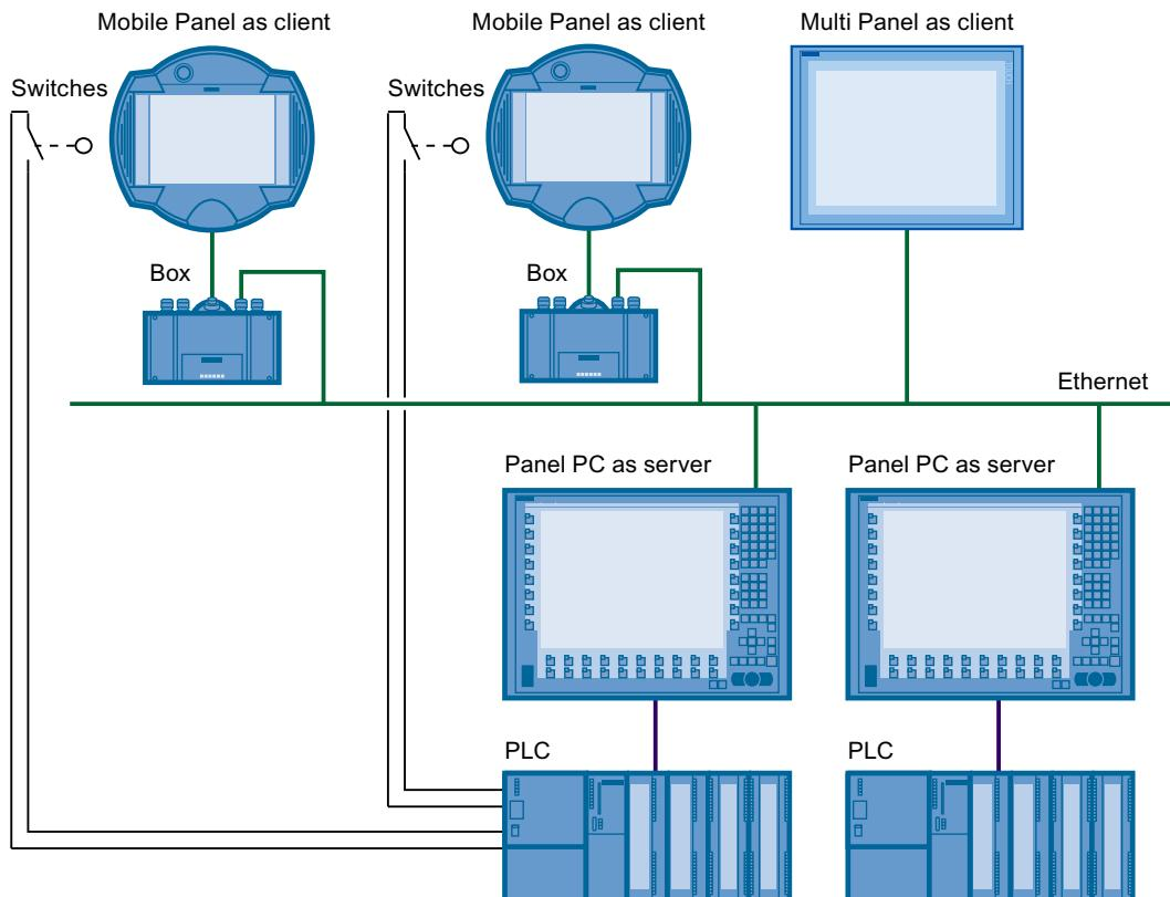
The nodes in the network communicate via Ethernet.
