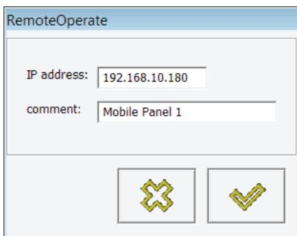
2. Enter in the "IP address:" box the physical address of the client which you want to add to the list of clients.
