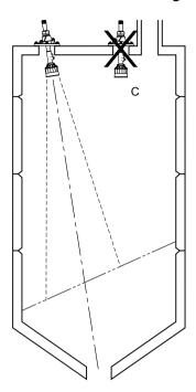
D - On fluid-like solids, aim transducer perpendicular to material surface.
