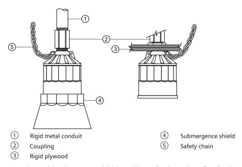
Transducer with submergence shield, used in applications where flooding is possible.
