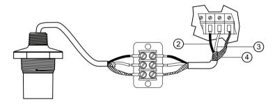
Extend cable using 0.823 mm<sup>2</sup> (18 AWG) shielded/twisted pair.
