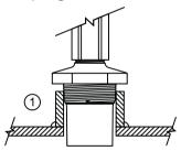
1) 2" coupling welded to tank top
