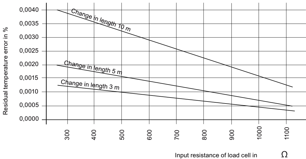
Figure 6-1 Residual temperature error for a load cell per 10 K temperature change when shortening or lengthening the connecting cable
