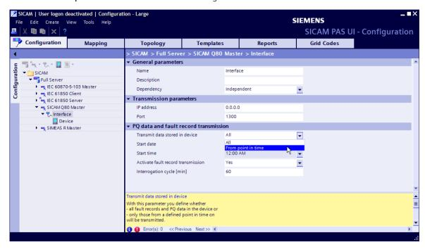
Figure 2-59 Transmitting Data from User-Defined Selection
