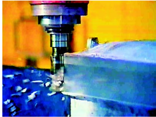
Roughing an external contour
