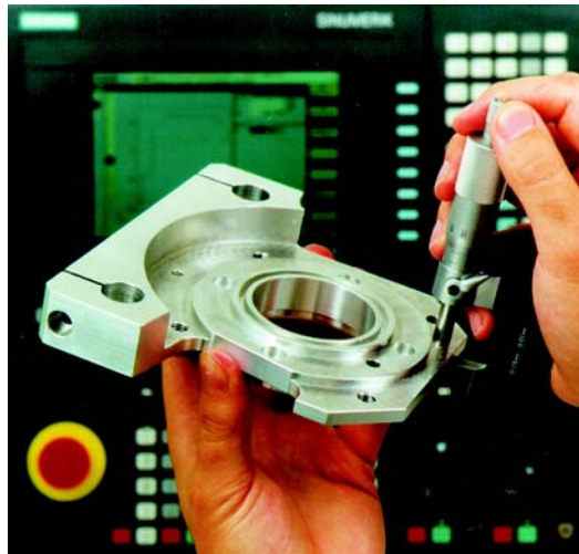
Measuring the plate thickness using an external micrometer
