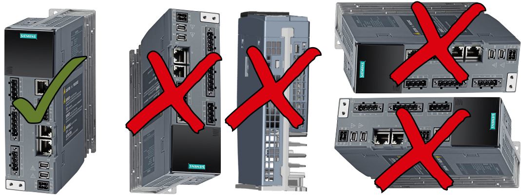
Figure 6-2 Mounting position of the converter
