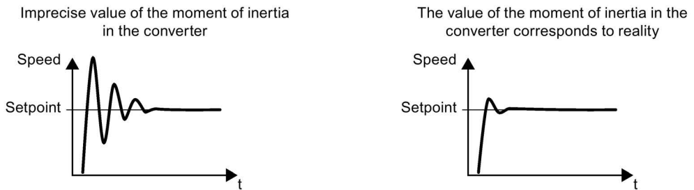
Figure 9-23 Influence of the moment of inertia estimator on the speed
