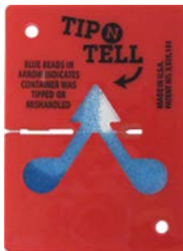
Figure 3-4 Tilt indicator tripped
