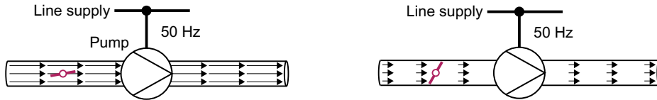
Figure 8-85 Flow control with pump and throttle connected to a 50 Hz line supply
