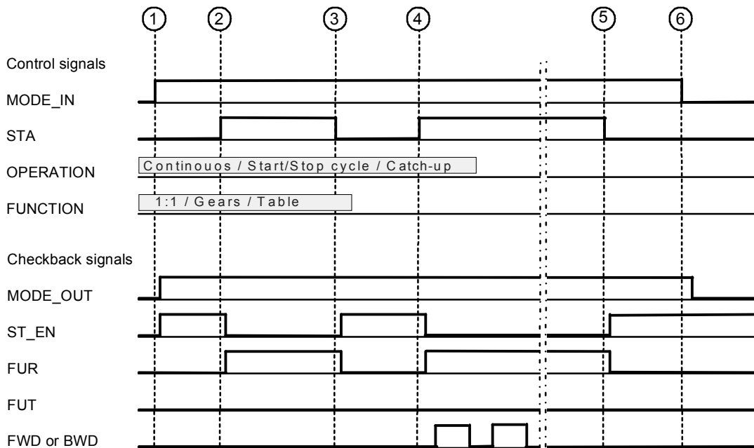
Fig. 10-2 Pulse diagram for synchronization mode
