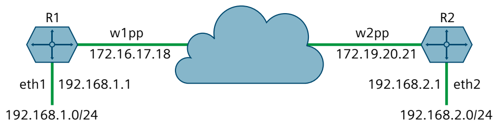
Figure 11.6 Example – GRE Tunnel Configuration
