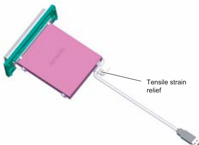
Figure 6-4 Strain relief for the cable
