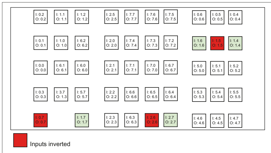
Figure 3-7 Inputs and outputs of the MCP 310 keyboard
