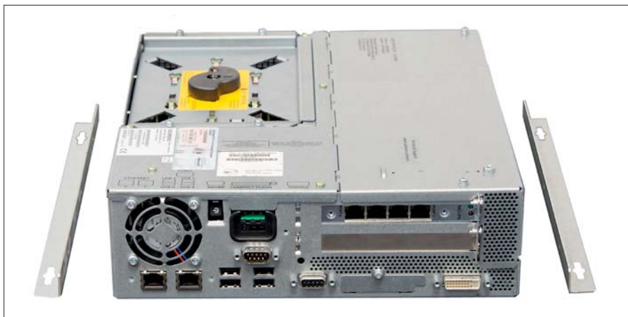
Figure 13-12 PCU 50.3 with mounting brackets for flat mounting
