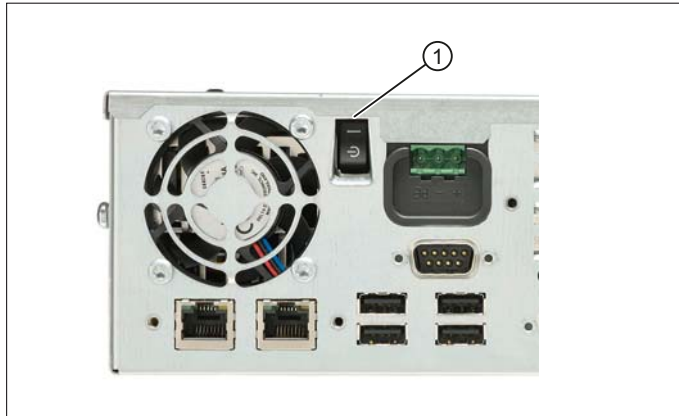
Figure 13-3 PCU 50.3 On/Off switch
