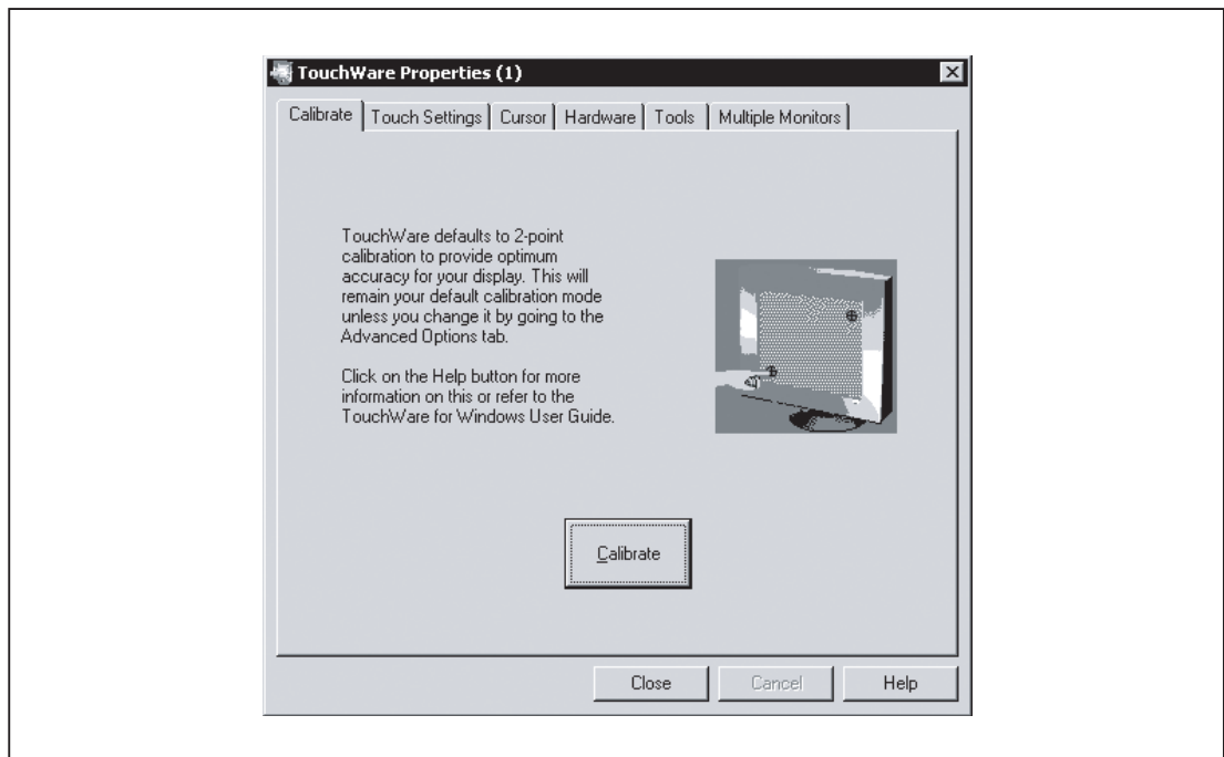
Figure 13-24 Menu for touch screen calibration (Touchware version 5.64 SR3)
