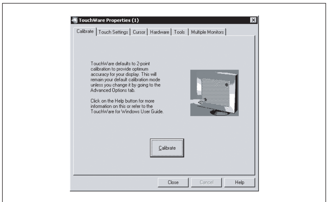
Figure 14-20 Menu for touch screen calibration (Touchware version 5.64 SR3)
