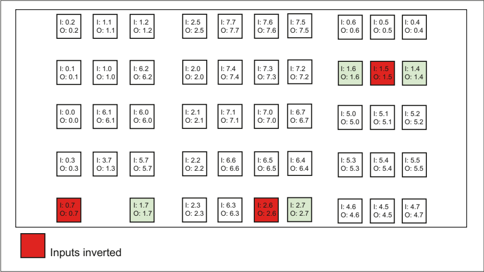
Figure 1-5 Inputs and outputs of the MCP 310C PN keyboard
