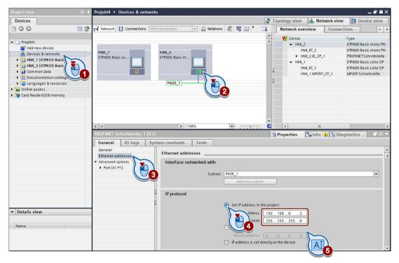
As an alternative, you can still set the IP address using the Control Panel of the HMI device or an DHCP server. In both cases, select the option "Get IP address another way" in WinCC (TIA Portal).
