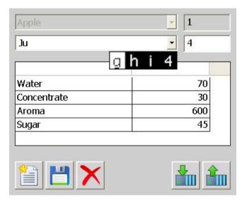
The following figure shows the alphanumeric input block for the KP400 Basic color PN:
