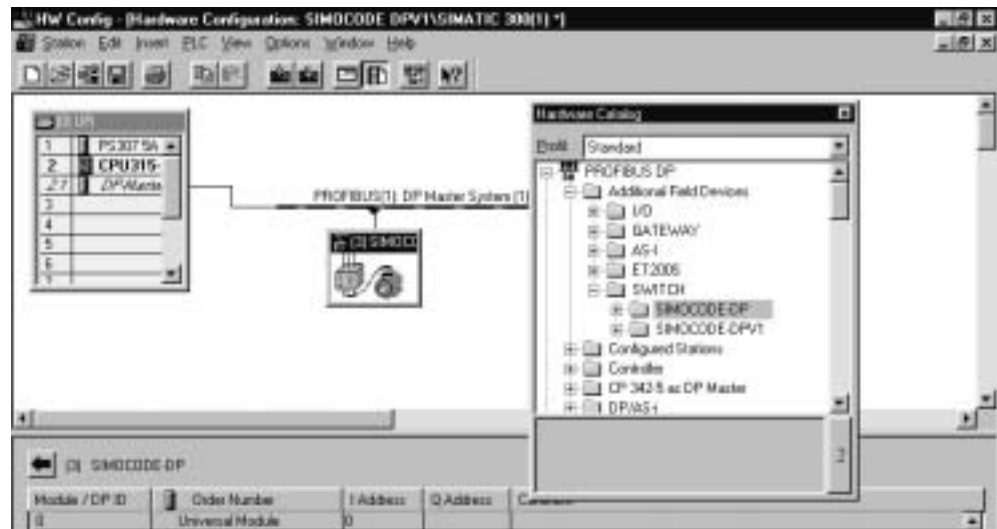
Selecting SIMOCODE-DP as a DP standard slave with HW Config (Hardware Configuration)
