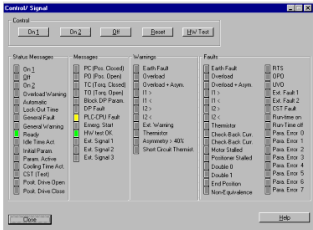
Fig. 49: Fast fault analysis with the "Control/Signal" mask
