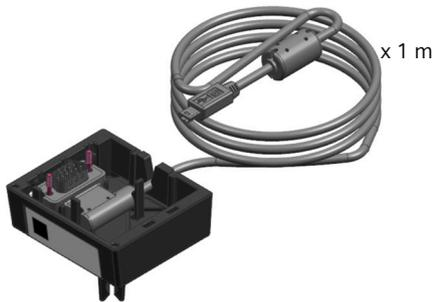
The SAM interface kit is designed with a rubber support and magnets, which allows you to easily mount the SINAMICS G120 Smart Access to the converter or remove it from the converter. The permissible operating temperature range for the SAM interface kit is from -10 °C to +60 °C. Vibration in operation fulfills Class 3M1 according to EN60721-3-3: 1995.
