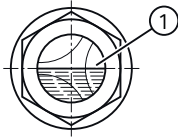
Figure 10-6 Oil level in the oil sight glass
