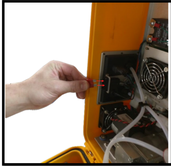
Figure 46: Install the New Fuse in the Fuse Holder
