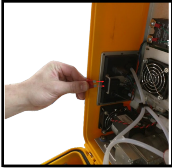
Figure 49: Install the New Fuse in the Fuse Holder
