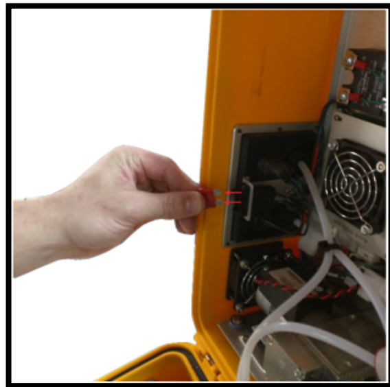
Figure 48: Remove the Fuse
