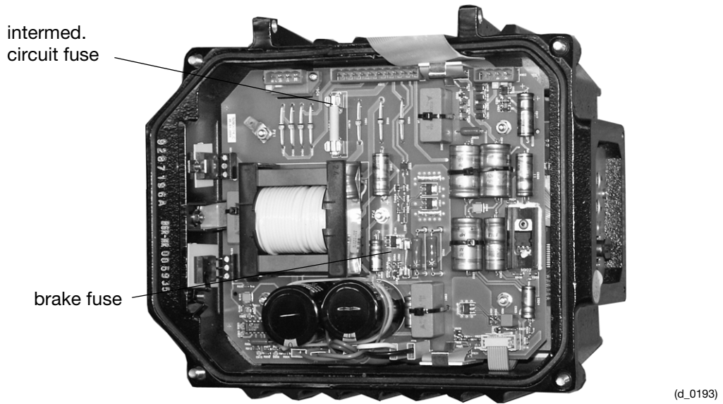
Fig. 35: Fuses in control-housing part
