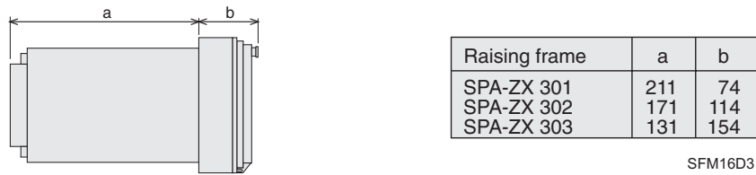
Fig. 8 Semi-flush mounting relay case (dimensions in mm)
