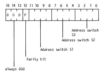
The address is set on the module by means of hex. code switches and can be read on the module front panel.
