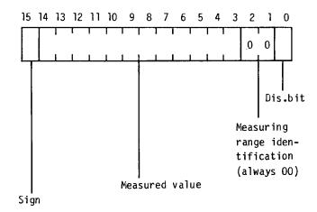
The disturbance annunciation output of the corresponding function unit is set by the fact that the disturbance bit is set or not in the respective data telegram.
