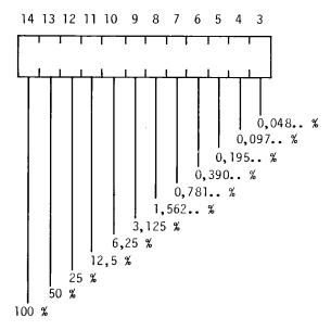
Adding the bits set to logic "l" yields the analog measured variable.
