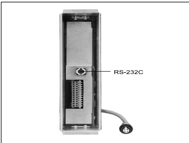
Fig. 4 Interface RS-232C on front panel with socket connector Z-16962
