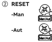
en In case of adjusting "RESET A", which means automatic reset after tripping, the motor may restart automatically. This automatic restart could injure persons and damage material.
