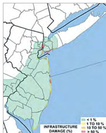
Figure A1-3 – Preliminary information on the percentage of power grid components damaged during superstorm Sandy [23]
