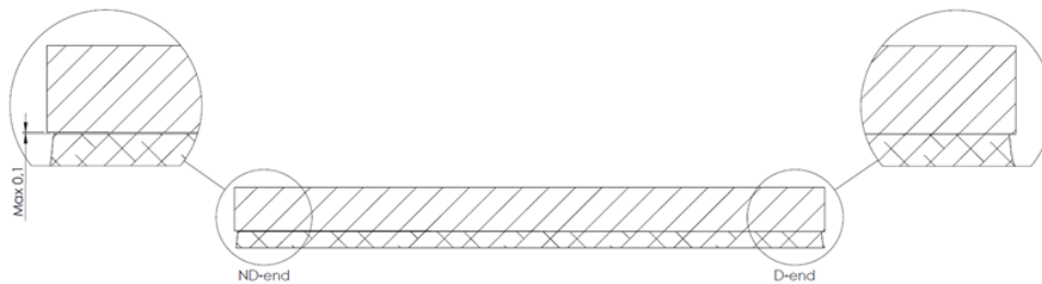
Figure 8. Max allowed height difference between D-end and ND-end.
