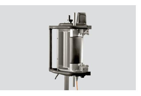
L&W Profile Cutter Advanced cuts sample strips directly from the machine reel. The samples are cut with precision to a fixed width and automatically wound onto a removable cylinder. The clean, wrinkle-free samples can be used for testing in L&W Autoline and L&W TSO Tester, or for routine testing in a quality control paper laboratory.
