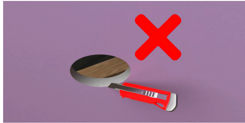
04 The box must be installed in the middle of the hole; the drilled hole must not be worked afterwards.
