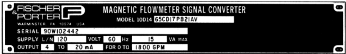
FIGURE 3-2. TYPICAL SIGNAL CONVERTER NAMETAG
