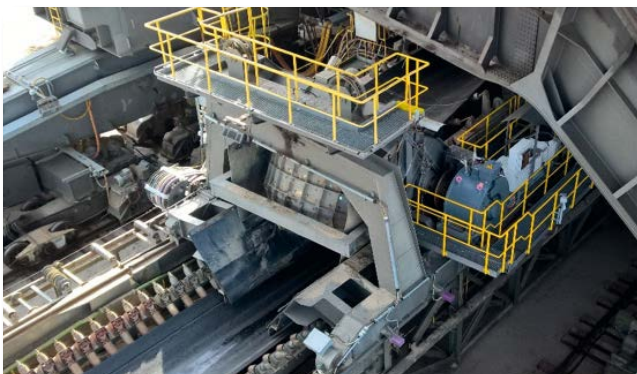
Figure 6: New ABB medium power GCD on excavator at the LEAG-owned Jaenschwalde lignite mine, close to Cottbus, Germany
