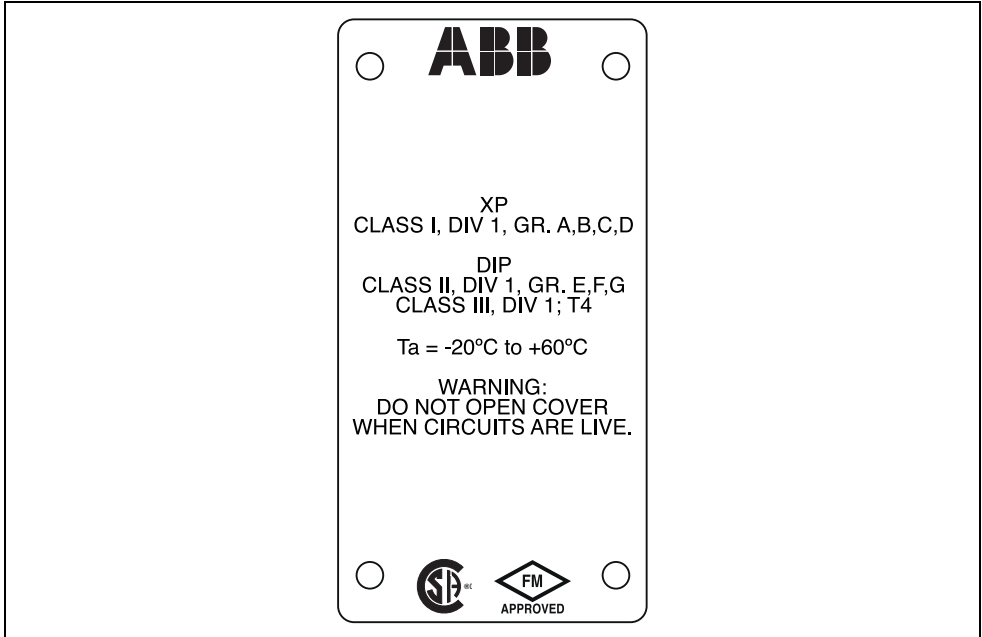
Fig. 3.9 Example of CSA / FM (Classes I, II and III; Div. 1 explosion- and ignition-proof) 'HazLoc' Label
