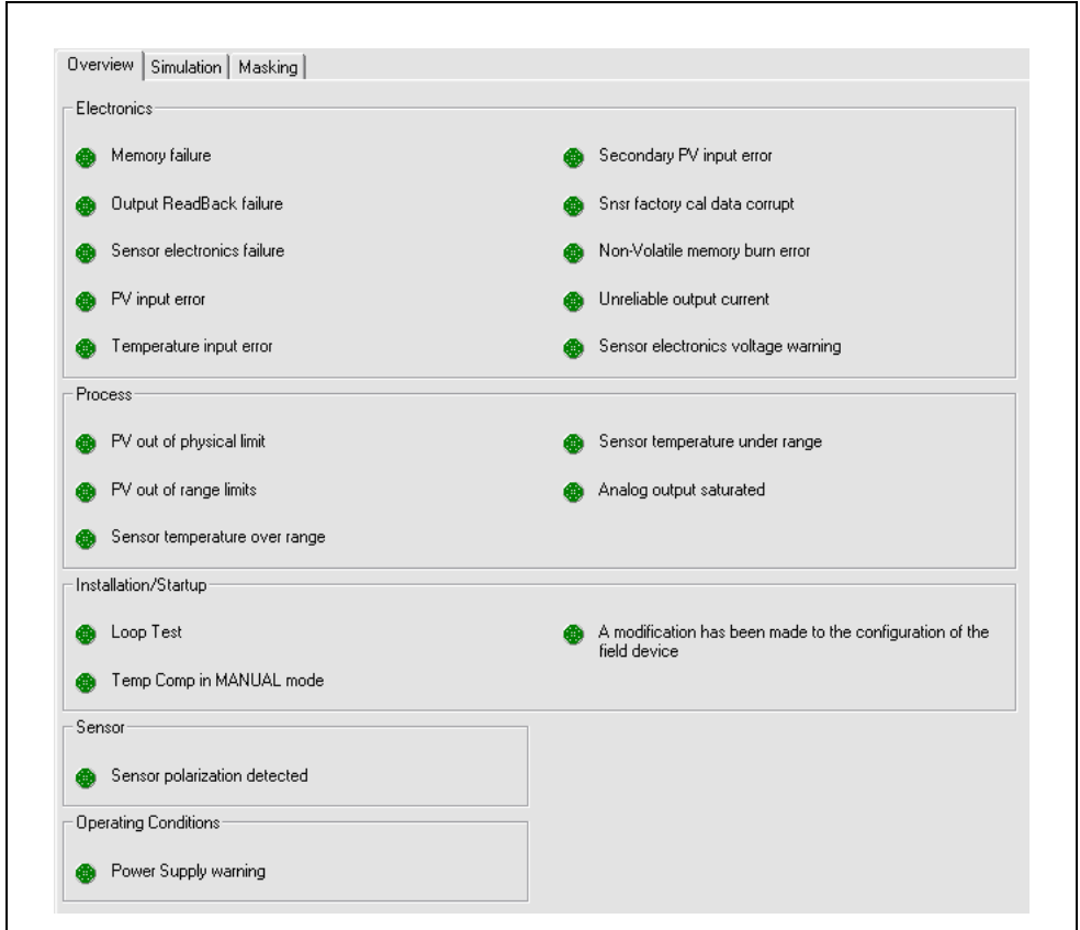
Fig. 8.2 ACA592 2-Electrode Conductivity Transmitter – Diagnosis Overview Screen
