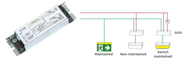
SI230 Changeover Relays are compact and east to install. When using these changeover relays, switched maintained emergency luminaires are energized whenever a local switched supply is present and automatically when a local sub-circuit failure occurs.
