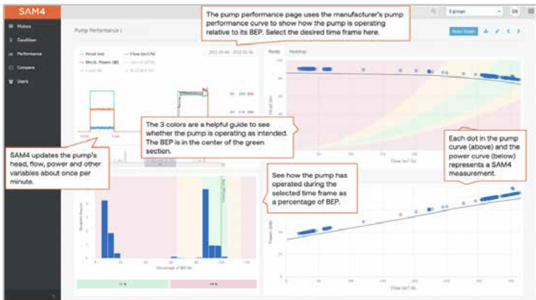
Sample real-time pump curve and performance metrics.
