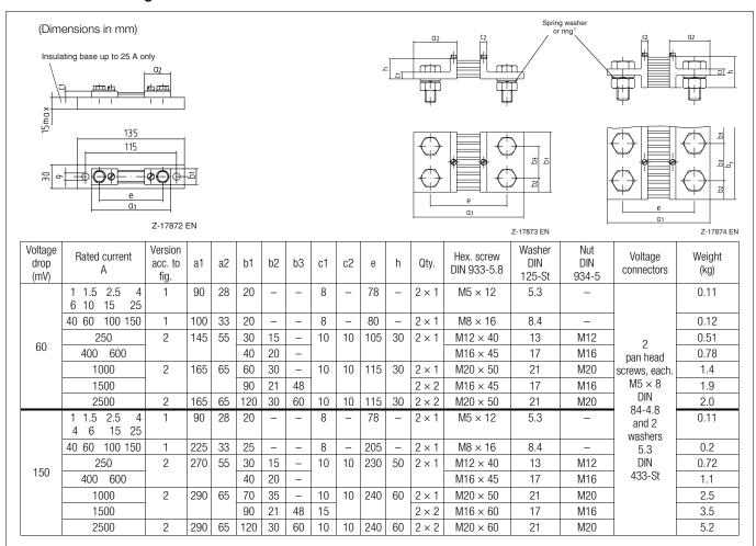
Details not provided should be selected as need be. Name of a shunt for 60 mV voltage drop and 25 A rated current: Shunt 60-25 DIN 43703
