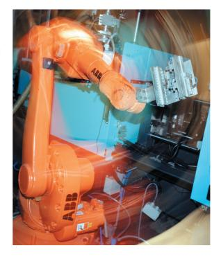
The Euromap/SPI input and output signals are easily configured in RobotWare, the robot controller software, using the provided IO-configuration files. In robot test mode when the machine is disconnected, the controller jumper plug is very useful.
