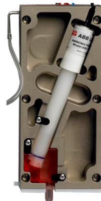
Figure 3 Electrode in temperature-controlled flow cell
