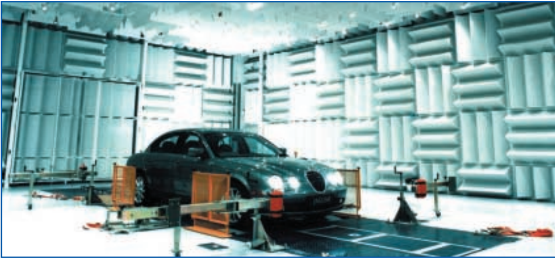
The car industry is a major user of test rigs, such as this one at Jaguar, manufactured by Froude Consine
