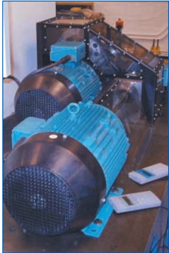
Multidrives involve two motors and drives, with one set motoring and the other generating; this unit is designed for the testing of cambelts
