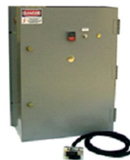
Figure 4.14 Breaker test cabinet
