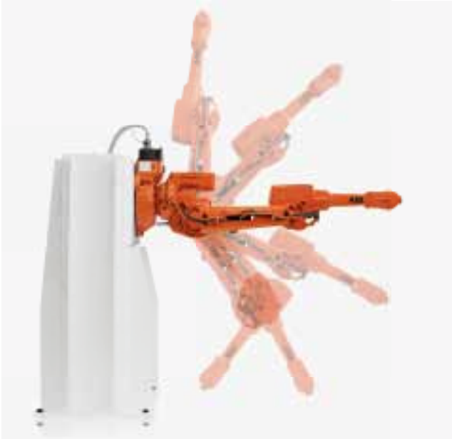
The IRB 2600, launched in 2010, has a payload capacity of up to 20 kg and an ultrawide working range. It has the smallest footprint in its class.
