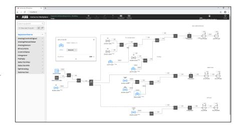
The main focus of ABB Process Model Engine is to offer a cost-efficient simulation product for automation systems. In an engineering phase where systems or control areas are integrated, it is beneficial to add more dynamic response to the simulation, so that manual response interactions towards the control system are reduced. Adding Loop Feedback to I/O and Device Feedback will provide a very efficient and realistic test environment for control system tests and early operator training.
