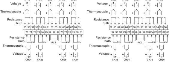
Note) For current input, connect an optional shunt resistance to a voltage input terminal.
